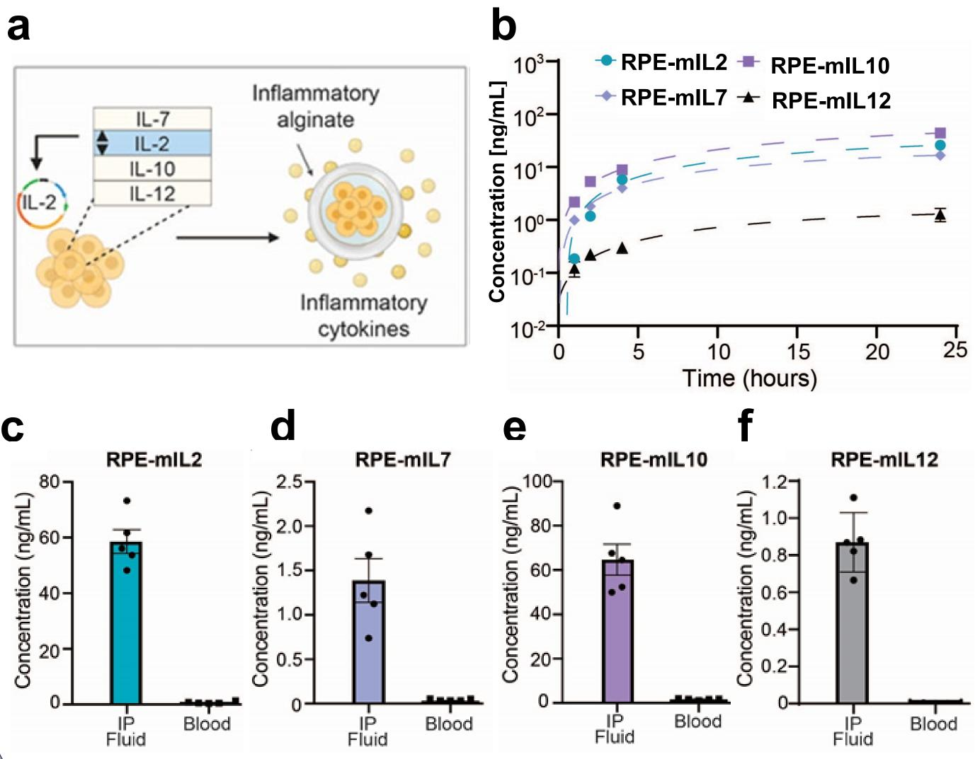
Above: a) Schematic of cell engineering and encapsulation approach. b) *In vitro* cytokine concentration at 1, 2, 4 and 24 hours (n=5). c-f) Cytokine concentration in IP fluid of mice 24 hours after implantation of RPE-mIL12, RPE-mIL7, RPE-mIL10, or RPE-mIL2 (n=5). Concentrations were measured using ELISA.
